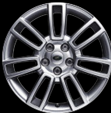
19 INCH TWIN 7-SPOKE ALLOYS 'STYLE 8' STANDARD HSE WHEEL – 255/55 R19
