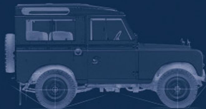
Series IIa Station Wagon (1961-1972) 1966 Electrical indicators become standard. 1968 Headlamps moved from radiator grille to wings.
