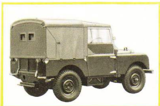
Semi-rear view of Land-Rover showing hood rear panel.
