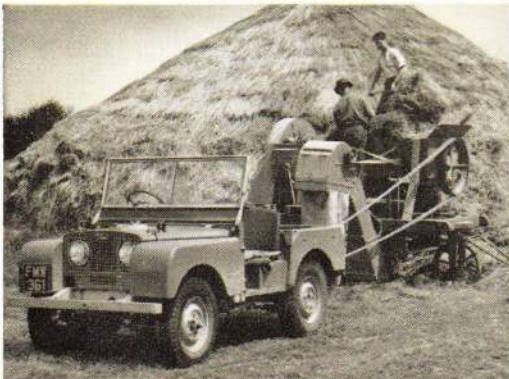
The Land-Rover operates Farm Machinery and tows it to the spot.
