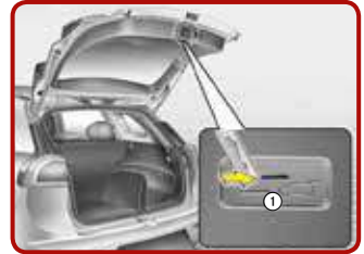
Emergency tailgate safety release [4]
