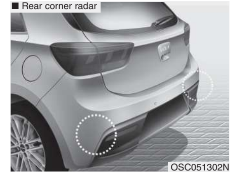
[A]: Rear Cross-Traffic Collision Warning operating range
