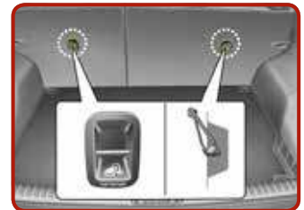
Securing with "Tether Anchorage" system [3]
