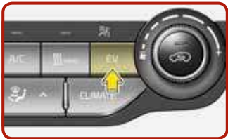
EV mode [EV-Guide] If you select the "EV" menu on the AVN home screen or press the "EV" button on the left side of the air intake control button, you can enter EV mode. The EV mode has a total of 5 menus.
