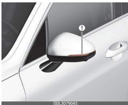
Light bulb position (Side)
