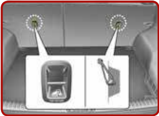
Securing with "Tether Anchorage" system [3]
