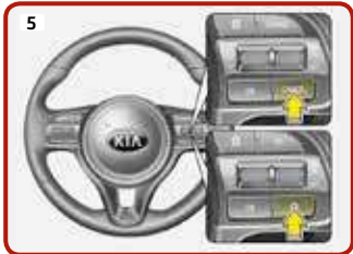
Cancel cruise control set speed by pressing the cancel button (CANCEL/O)
