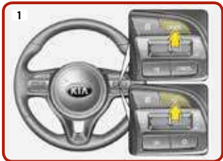
Cruise control system* [5] ON-OFF button (CRUISE/ON-OFF) to activate cruise control system
