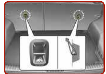
Securing with "Tether Anchorage" system [3]
