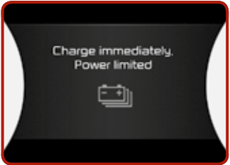
Charge immediately [EV-Guide] High voltage battery level ~3% or less
