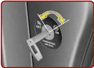
Passenger's front air bag ON/OFF switch* [3]
