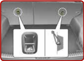
Securing with "Tether Anchorage" system [3]
