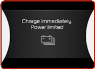
Charge immediately [EV-Guide] High voltage battery level ~3% or less
