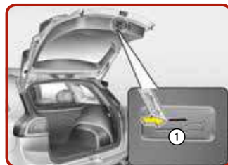
Emergency tailgate safety release [4]
