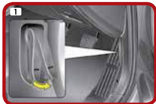
Opening the bonnet [4] Pull the release lever to unlatch the bonnet.
