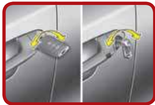
Operating door locks from outside the vehicle [4]
