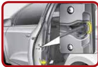
Locking doors in case of an emergency [4]
