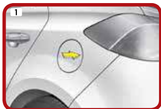
Opening the fuel filler lid [4] Press the center edge of the lid when all doors are unlocked.
