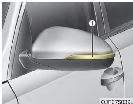
(1) Side repeater lamp (LED type)
