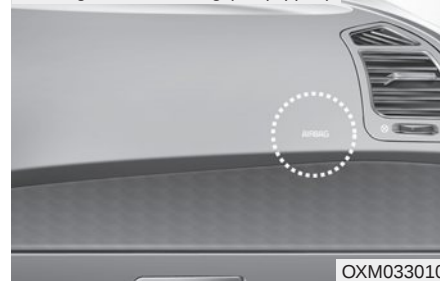
Passenger's front air bag (if equipped)
