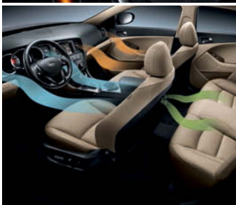
DUAL-ZONE AUTOMATIC TEMPERATURE CONTROL* Driver and front passenger can adjust their own temperature setting for individual comfort zones. These two levels are blended for those in the rear.
