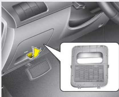
Inner fuse panel
