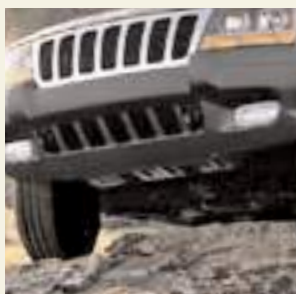
An available front suspension skid plate helps prevent underbody damage.
