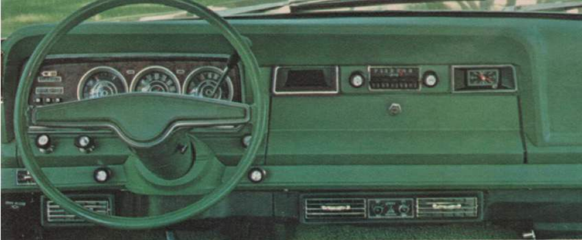
Newly-designed instrument panel, with standard direct-reading oil and ammeter gauges.
