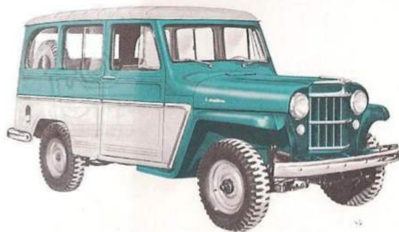
'JEEP' 4WD UTILITY WAGON carries 1,000 lbs. cargo or six passengers. Newly styled inside and out, with 1-piece windshield and 1-piece tailgate glass. Choice of 4 or 6-cylinder engines.
