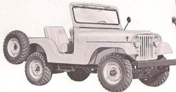
'JEEP' UNIVERSAL CJ-5 loads 1,476 lbs. of cargo. Modern design combines with traditional 'Jeep' ruggedness. Optional metal and fabric tops. F-Head "Hurricane" engine.
