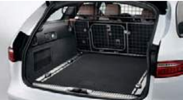
Luggage Guard** T2H31273 The luggage compartment partition is designed to prevent cargo from entering the passenger compartment.
