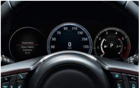
12.3" Full Digital Instrument Panel with virtual dials
