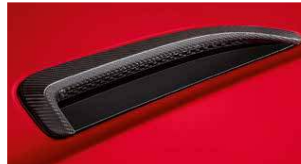
Carbon Fiber Hood Louvers* T2R5275PEC - Left Side RWD T2R5274PEC - Right Side RWD T2R16704 - Left Side AWD T2R16703 - Right Side AWD
