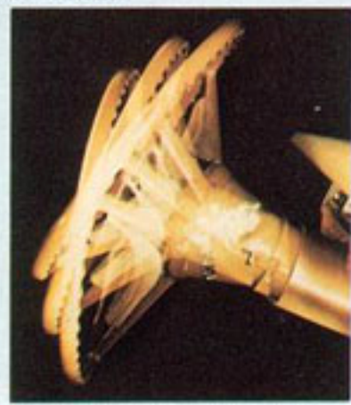
Seven-position tilt steering wheel. Adjustable so a driver can select a comfortable position; easier to enter and exit.
