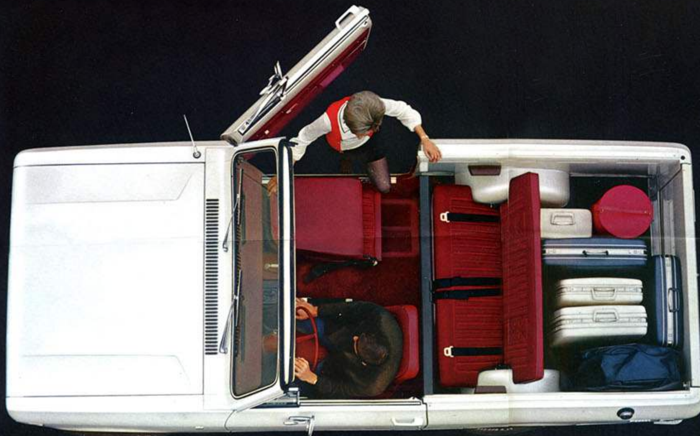
On the level. Floor and door frame are same height. No stepping down into a well or up to get into the back seat.
