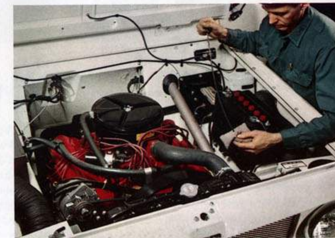
Routine servicing is a snap — All three Scout engines are nestled in a large, low compartment. Distributor, plugs, coil and air filters can be reached without groping. Oil and other routine checks can be made from the front.
