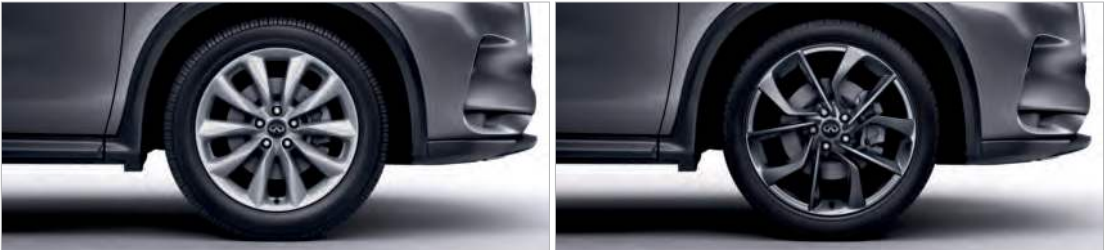
19 X 7.5-INCH SILVER-PAINTED ALUMINUM-ALLOY WHEELS 20 X 8.5-INCH DARK-PAINTED ALUMINUM-ALLOY WHEELS*
