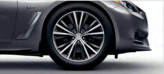
19 X 9.0-INCH ALUMINUM-ALLOY WHEELS
