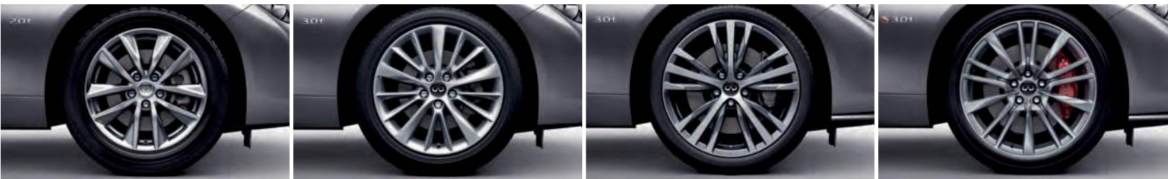
17 X 7.5-INCH SPLIT 5-SPOKE ALUMINUM-ALLOY WHEELS 18 X 7.5-INCH ALUMINUM-ALLOY WHEELS** 19 X 8.5-INCH SPORT-DESIGN TRIPLE 5-SPOKE ALUMINUM-ALLOY WHEELS** 19 X 9.0-INCH FRONT, 19 X 9.5-INCH REAR STAGGERED ALUMINUM-ALLOY SPORT WHEELS*
