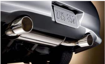
SPORT MUFFLER The polished, stainless steel muffler showcases a deeper, throaty exhaust tone. Larger-diameter exhaust tips help let it breathe and the muffler is fabricated with TIG welds not only for appearance but for strength and longer life.
