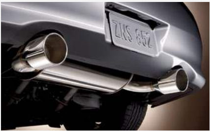
SPORT MUFFLER The polished, stainless steel muffler showcases a deeper, throaty exhaust tone. Larger diameter exhaust tips help let it breathe and the muffler is fabricated with TIG welds for a precision-crafted appearance.
