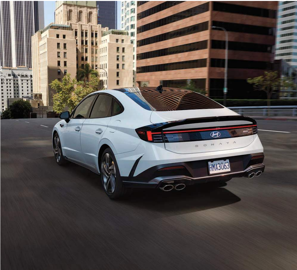
N Line quad-outlet dual exhaust system and LED combination taillights
