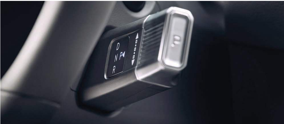
Steering column-mounted Shift-by-Wire gear shifter
