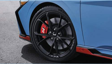
19” forged wheels and 14.2” front brake rotors
