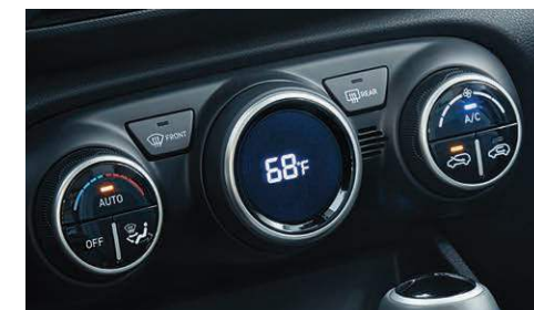
Automatic temperature control
