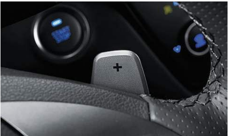
Regenerative brake-level control paddles
