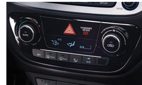
Automatic temperature control
