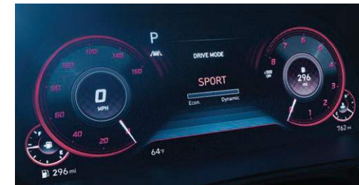
12.3" instrument cluster display in Sport mode
