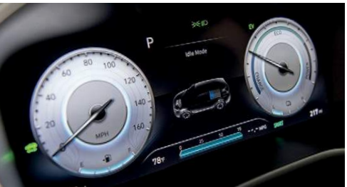
12.3" digital LCD instrument cluster
