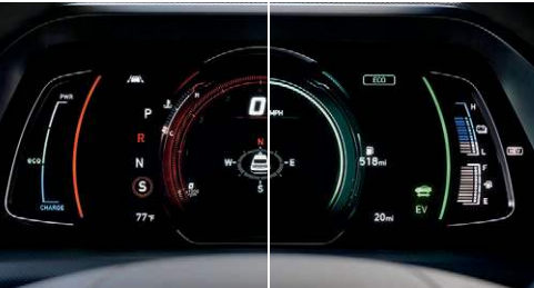
7” LCD instrument cluster (Sport/Normal modes)
