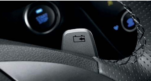
Regenerative brake level control paddles
