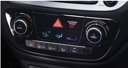
Automatic temperature control
