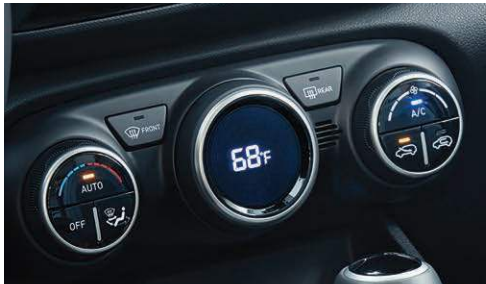
Automatic temperature control
