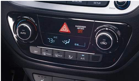
Automatic temperature control
