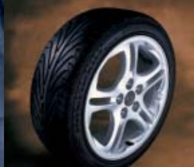
The GT V6 has standard 17-inch aluminum alloy wheels 1 with 215/45 Michelin® tires that provide quick handling.
