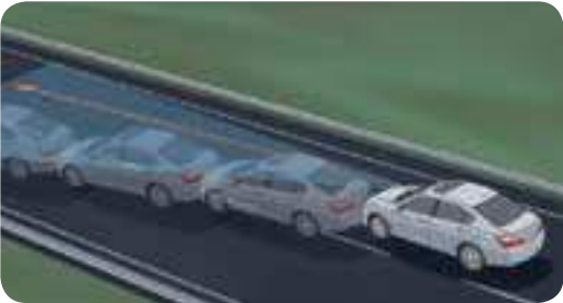
LANE DEPARTURE WARNING (LDW) 9 A small camera searches for lane markings on the road. If it detects the driver making an unindicated lane departure, visual and audible alerts will signify the departure. (EX-L and above)
