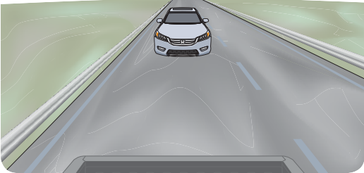
ADAPTIVE CRUISE CONTROL (ACC) 11 ACC electronically regulates your following distance in Adaptive Cruise Control mode, accelerating or decelerating depending on how close you are to the vehicle detected in front of you. (Touring)
