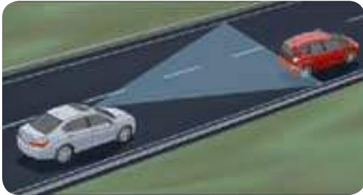
FORWARD COLLISION WARNING (FCW) 10 The FCW system can sense the presence of vehicles in front of you, and if it calculates that you're at risk of a collision with a detected vehicle, it activates audible and visible alerts. (EX-L and above)
