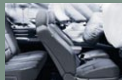
Front airbags inflate and deflate in a fraction of a second.
