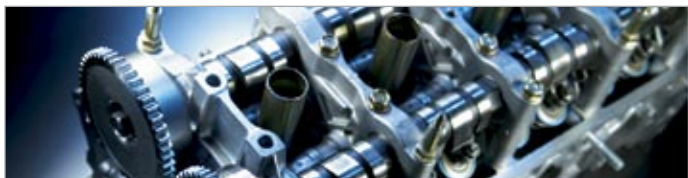
❖ 3-rocker i-VTEC for a broad powerband.
