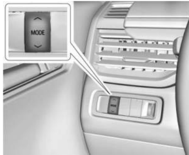
Driver Mode Control Switch
