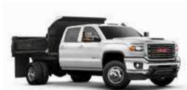
SIERRA HD CREW CAB CHASSIS CAB with dump body upfit. 3
