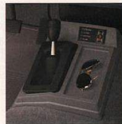
Insta-Trac transfer case provides shift-on-the-fly convenience.
