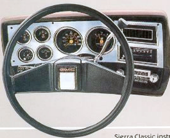
Sierra Classic instrument cluster with needle-type gauges to indicate charging system voltage plus engine temperature and oil pressure
