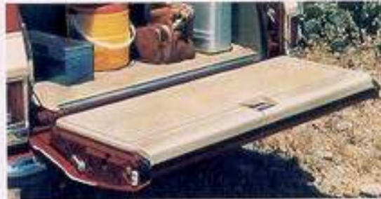
Wagon-type tailgate offers available power drop glass, with or without electric defogger.
