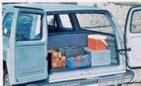
Panel-type rear doors have fixed, tinted glass; opening is 37" high by 59.6" wide. Power door lock available.
